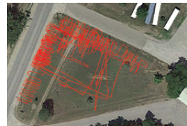
Depth slices from GPR Lines
