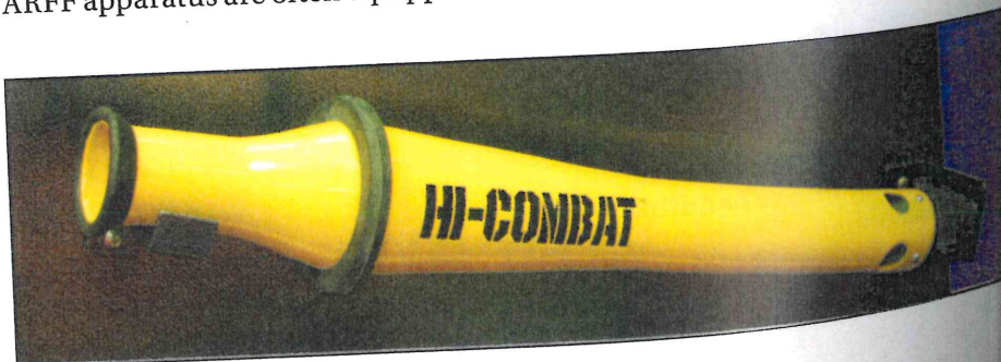
Figure 14.28 Air-aspirating nozzles induct air into the foam solution allowing for maximum expansion of the foam.
