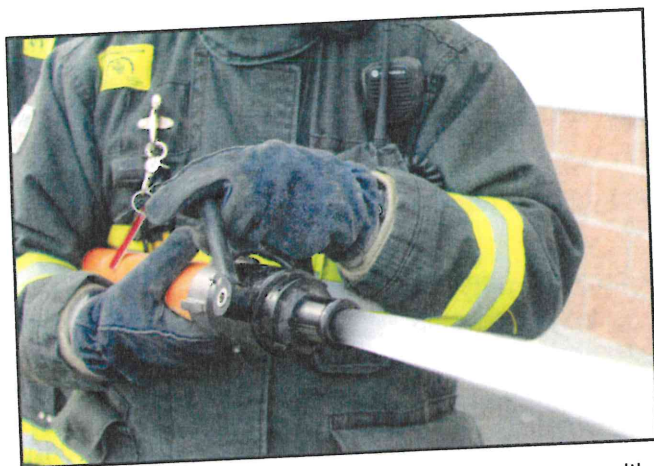
Figure 14.26 A smooth bore nozzle provides a stream with excellent reach. Courtesy of Shad Cooper/Wyoming State Fire Marshal's Office.
