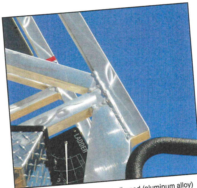
Figure 16.6a An example of a welded (steel) truss.
