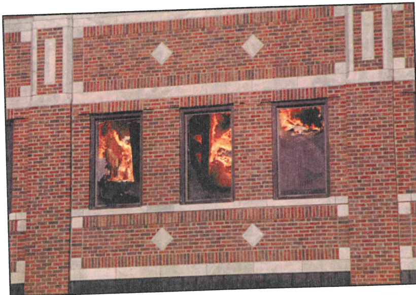
Figure 20.39 Combustible interior items may begin to burn if exposed to radiant heat.
